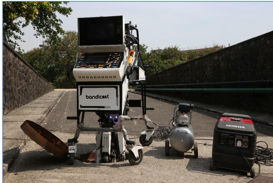
Mechanical Cleaning of sewers chambers and septic tanks using Robotics; Department of Atomic Energy
